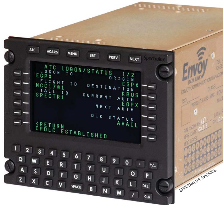
Envoy includes three integrated avionics modules: a CMU, VDR and a MCDU.
