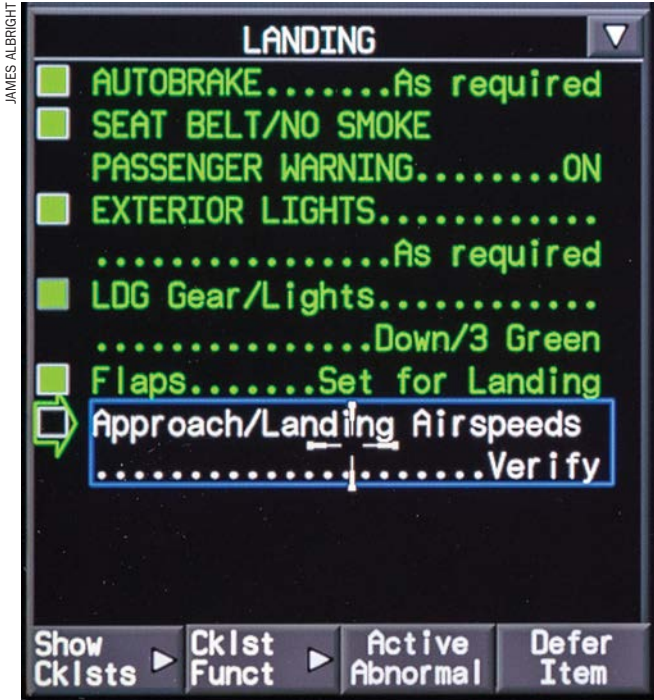
The GVII's electronic before-landing checklist, with the first five items automatically completed
