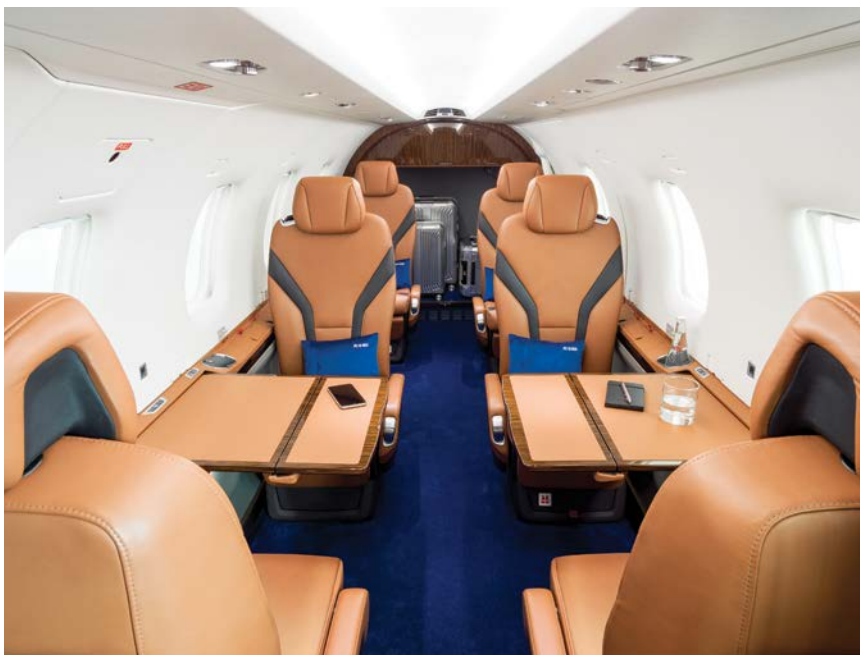
The 6 + 2 seat exterior interior is a $455,000 option. New chairs recline fully to create lie-flat berths. Quick release chair mounts allow interior to be reconfigured for cargo in less than 10 minutes. (Rearmost +2 seats not shown.)
